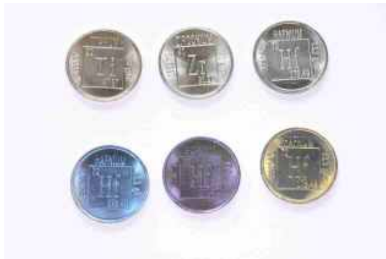
top row - coins of elements Titanium, zirconium and hafnium bottom row - anodized coins of hafnium in varying colours.
