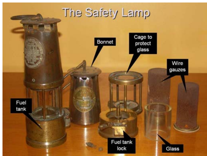
The anatomy of miner's safety lamps, from his collection, and as shown in the presentation; Tony Forsyth (Qld)
